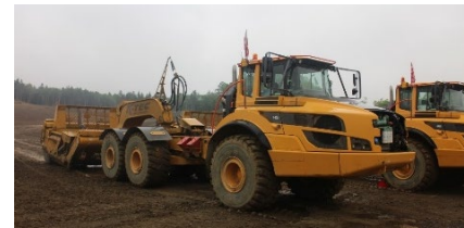
"Scraper", a heavy machine that can handle excavation, loading, transportation, and laying earth
