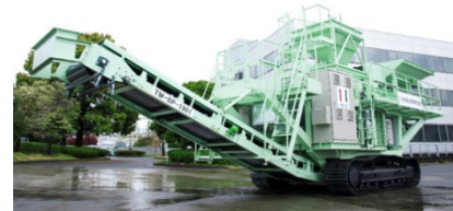
Self-propelled soil improvement machine of Rotary Crushing and Mixing Method (Twister Method)
